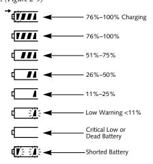
Figure 2-9 Battery Level Indicator
